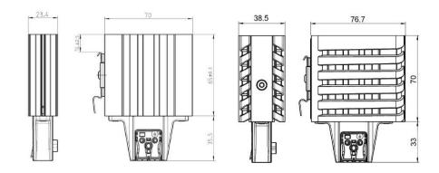
Danger! Heating may only be installed with a distance of 50mm to the side and above 100mm to the next component.
