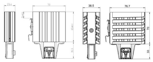
Danger! Heating may only be installed with a distance of 50mm to the side and above 100mm to the next component.
