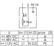
(1) Special voltages e.g.: 12V AC/DC, 24V AC/DC, 48V AC/DC, 115V AC, 400V AC available upon request.
