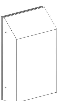
Stainless steel hoods must be used on the flat surface of Type 1, 2, 3, 3X, 3R, 3RX, 3S, 3SX, 4\*, 4X\*, 5, 12, 12K or 13 enclosures
