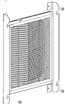
Fix the mounting brackets using the screws / washers / nuts provided.
