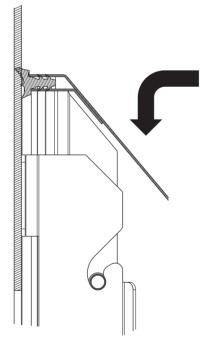
Assemble the hood by pushing towards the panel and then firmly downwards.
