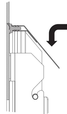
3. Assemble the hood by pushing towards the panel and then firmly downwards.
