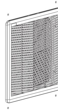
1. Drill 4 holes centred around the filter fan.
