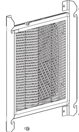
2. Fix the mounting brackets using the screws / washers / nuts provided.
