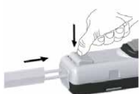
Pushfit connector ø AWG 22 - 16 ø AWG 22 - 18
